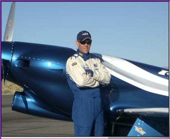
He placed second in the Silver Class in 2003 in his Glasair III, and in 2005 finished third in his new NXT "Relentless." Nemesis NXT (Neoteric eXperimental Technology) is a two-place, retractable gear, single engine, kit airplane of very sleek aerodynamic molded carbon fiber construction. Kevin's Nemesis NXT is powered by a Lycoming TIO-540-NXT engine and a special racing Hartzell 3-Blade Propeller.
