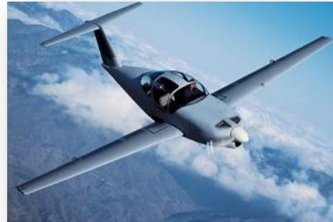
Peter went on to design and build a replacement, the four-place, all-composite *Melmoth 2*, with retractable gear and a 200hp turbocharged engine.
