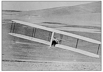
1902 Model B glider used as the basis for the Wright's patent applications
