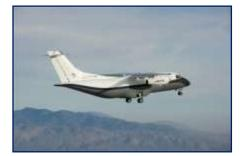
first test flight June 2 from Air Force Plant 42 in Palmdale, Calif. The ACCA is proof of concept technology demonstrator for advanced composite manufacturing processes in a full-scale, certified aircraft. It was developed by the Air Force Research Laboratory and Lockheed Martin.
