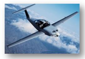
Peter went on to design and build a replacement, the four-place, all-composite *Melmoth 2*, with retractable gear and a 200hp turbocharged engine.
